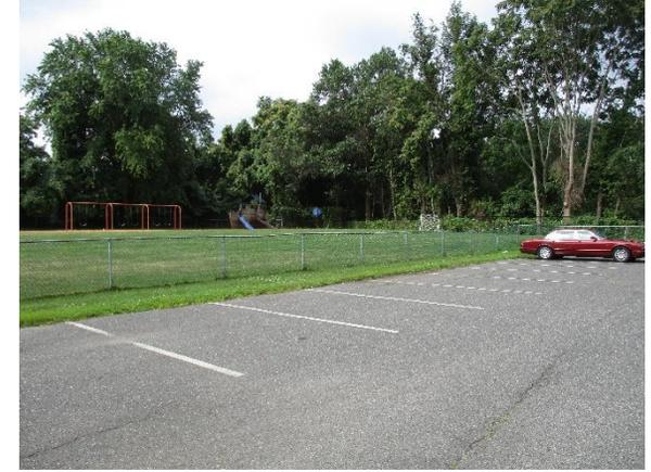
Rain gardens can be constructed at several locations to capture, treat, and infiltrate roof runoff. An additional rain garden can be installed to manage runoff from the driveway. A row of parking spaces can be replaced with pervious pavement to capture and infiltrate parking lot runoff. A preliminary soil assessment suggests that the soils have suitable drainage characteristics for green infrastructure.
