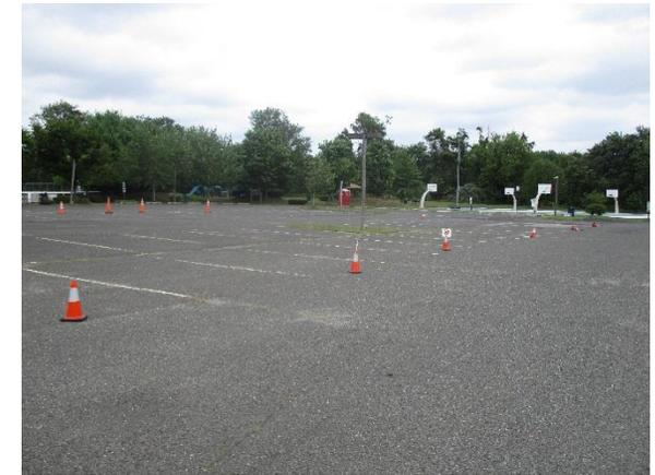
The recreation center's parking lot drains to the north. Parking spaces can be converted into pervious pavement to capture and infiltrate this runoff. The building already has disconnected downspouts that flow onto the grass and then into catch basins. Rain gardens can be installed to capture, treat and infiltrate this runoff. A preliminary soil assessment suggests that the soils have suitable drainage characteristics for green infrastructure.
