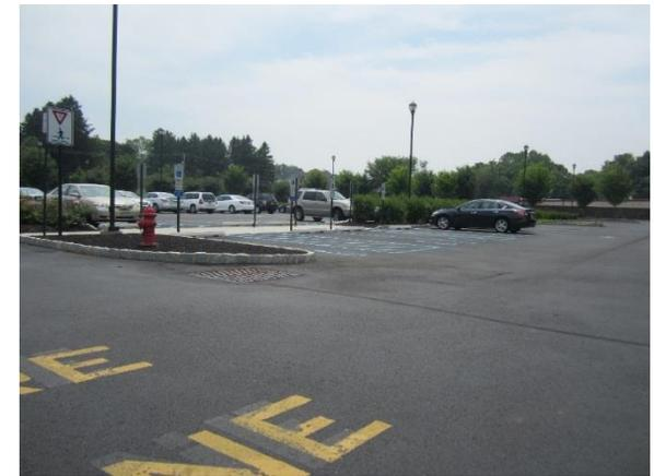
Runoff from the roof and parking lot appears to drain into an existing bioswale. A rain garden can be constructed in the turf grass area south of the Worship Center to capture, treat, and infiltrate some of this runoff. A preliminary soil assessment suggests that more soil testing would be required before determining the soil's suitability for green infrastructure.
